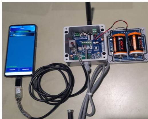
Figure 6-6 EWN-01V VW node connected to Android phone with FTDI cable via OTG adaptor
